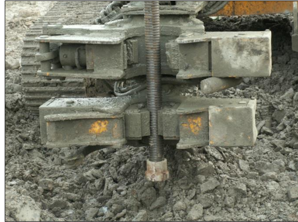
Figure 21. Jaw clamps for rod release
