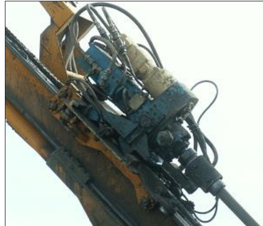
Figure 23. Heavy drifter for larger hollow bars
