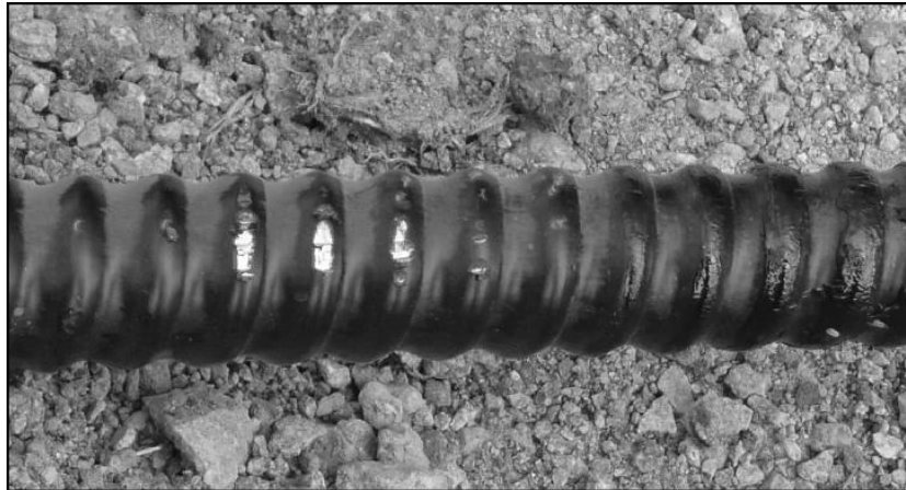
Figure 4. Duplex coating on hollow bar, showing exposed galvanized coating on top of the thread.
