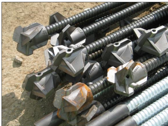
Figure 13. Two-stage retroflush drill bits
